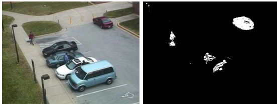
Fig. 2. A frame from a parking lot sequence and its corresponding foreground regions detected using background subtraction. Here, parked cars introduce significant occlusion and door openings lead to many false alarms.
